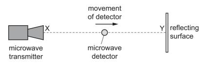
A microwave detector is moved steadily in a straight line from X to Y. A series of maxima and minima of intensity is obtained. The distance between adjacent maxima is 1.5 cm.
