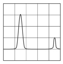
The time interval between two adjacent peaks of the waveform is 0.006 s.
